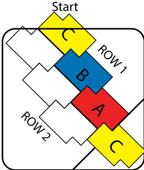
Start with either tool A/B/C from joint line and/or edge of form.
