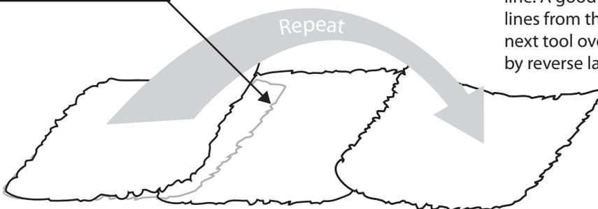
\*Note: Do not stamp up to edge to avoid seam line. A good method to get rid of seam lines from the previous spot is to stamp next tool overlapping the previous spot by reverse lapping them
